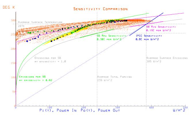
The small red dots are one month of data for each 2.5 degree slice of latitude from pole to pole along the input path plotting the average surface temperature, T, along the Y axis
